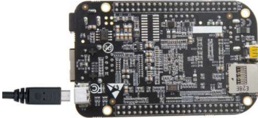
Figure 3. USB Connection to the Board
