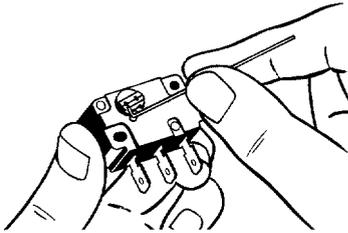
2. Push the lever down in the direction of the groove in the rotary disc.
