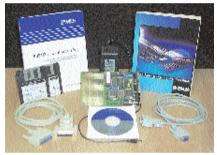
This system is aimed at developers looking to evaluate/program the high speed Dallas 87C520 microcontrollers. The kit is based around a 'Universal 8051 Monitor Module' which allows user code to be downloaded into external RAM and then single-stepped under PC control using the Keil 'dScope' debugger. The system is supplied with an advanced Windows Integrated Development Environment (IDE), Keil C51 Compiler, Assembler and Debugger. This makes it ideal for evaluation and small projects.
