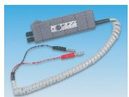
A high accuracy multimeter probe for differential/gauge pressure measurement of non-corrosive, non-ionic liquids and gases. Pressure can be applied to both or either of two ports to measure differential or gauge pressures. The unit has internal temperature compensation.
