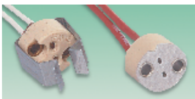
GU5.3 H = 22.2 (inc. clip), W = 19.2, D = 17 2 mtg holes Dia 3.6 @ 12 ctrs Lead Length = 140 GX5.3 H = 16.8, W = 18.6, D = 10.3 2 mtg holes Dia 4 @ 12 ctrs Lead Length = 160
