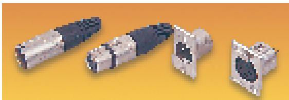
Free plug L = 69, Dia = 19.2 Free socket L = 72, Dia = 19.2 Cable entry = 2.8 – 8 Panel plug H = 36.7, W = 22 Panel cut out A Panel socket H = 36.7, W = 27 Panel cut out C
